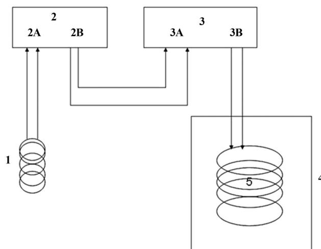
**Figure 1.** Experimental apparatus and assembly. 1—Source signal coil, 2—Electronic amplifier, 2A—Input signal in the electronic amplifier, 2B—Output signal from the electronic amplifier, 3—Wave generator, 3A—Input signal in wave generator, 3B—Output signal from wave generator, 4—Cell incubator, 5—Target coil. Used with permission of the journal of alternative and complementary medicine.
